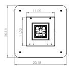
RETROFIT FOR 10" OR LARGER RECESSED ENCLOSURE FROM EXISTING LUMINAIRE. (NO ELECTRICAL ENCLOSURE PROVIDED)
