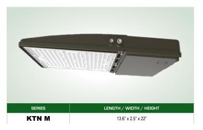
**ELECTRICAL SYSTEM** — Available in up to a 39,000 nominal lumens in most optical distributions with either 4000K Neutral White or 5000K Cool White color temperatures. Universal input votltage 120-277Vac, 50/60Hz; 347/480Vac. Operating temperature range -40°C to 40° C.
