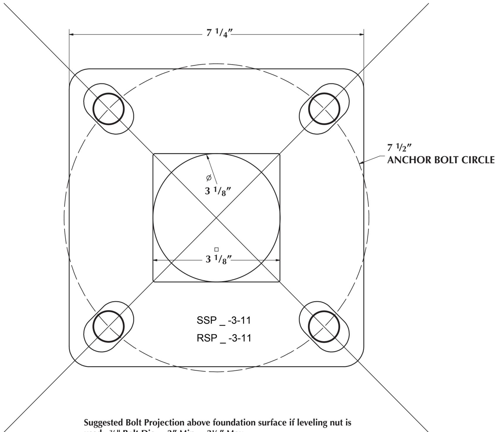
**Suggested Bolt Projection above foundation surface if leveling nut is used: 3/4" Bolt Dia. – 3" Min. – 3 1/2" Max.**
